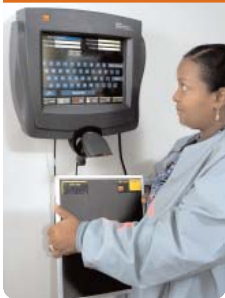
Marielynda Richeme, RT (R), uses a Kodak DirectView remote operations panel associated with a Kodak DirectView CR 900 system to read the bar code on an image cassette. The panels, which are located in examination rooms, allow technologists to enter patient and exam information and perform image reviews without leaving the room.
